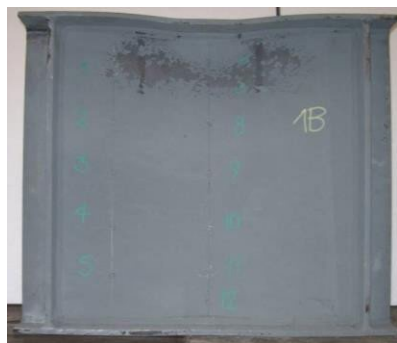
Fig. 16: Out-of-plane displacements of the web girder in the sample 5B
