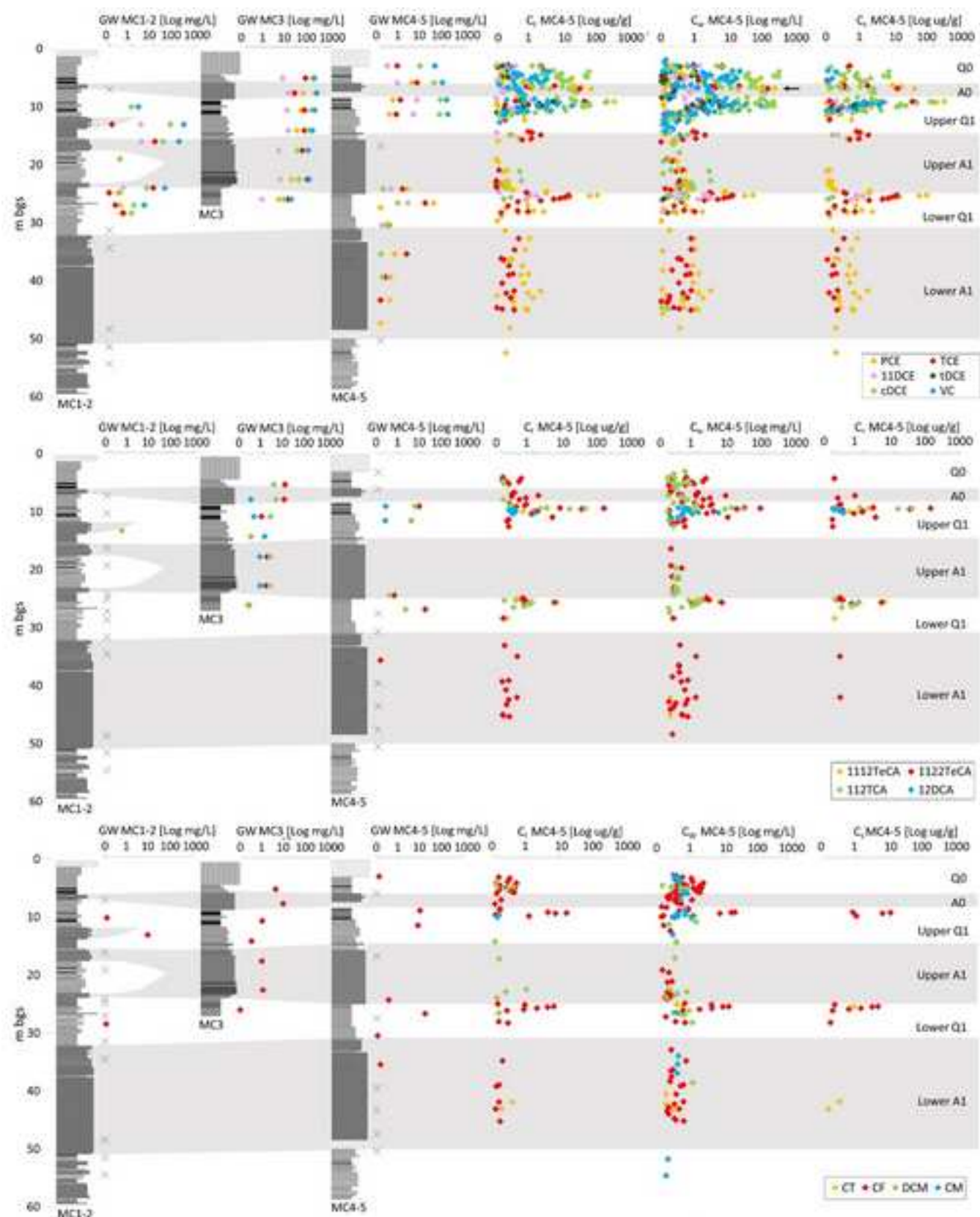
Figure 4: Vertical distribution of chloroethenes (a), chloroethanes (b) and chloromethanes (c). From left: concentrations from groundwater samples (GW; Log mg/L - only concentrations > 0.1 mg/L are plotted for graphical reasons (black crosses indicate GW samples with concentration < 0.1 mg/L for all the analyzed compounds); total concentrations in sediment samples along profile MC4-5 (Ct, Log \mu\text{g/g} - only concentrations > 0.1 \mu\text{g/g} are plotted for graphical reasons); estimated pore water concentrations from phase partitioning (Cw; Log mg/L - only concentrations > 0.1 mg/L are plotted for graphical reasons); estimated sorbed mass concentrations from phase partitioning (Cs; Log \mu\text{g/g} - only concentrations > 0.1 \mu\text{g/g} are plotted for graphical reasons). The one sample with estimated pore water concentration of PCE most likely higher than effective solubility is highlighted with a black arrow. The concentration database is in Tables S2 and S3 of the SM.
