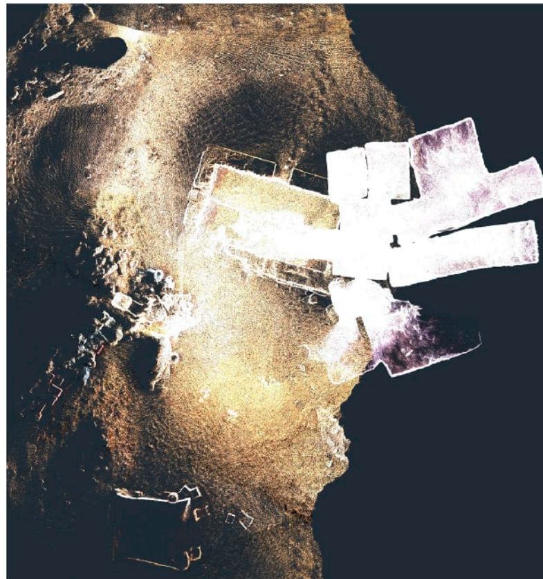
Figure 10. Top view of a portion of the point cloud for the tomb AGH032 showing both above and below-ground surface in “X-Ray” mode.
