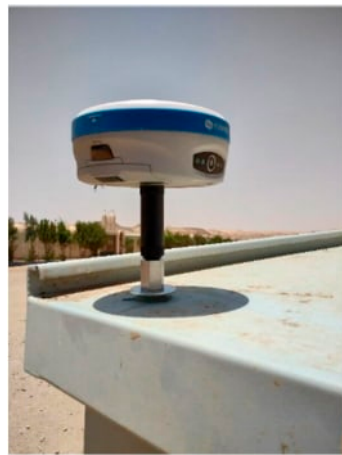
Figure 2. The fixed reference GNSS antenna mounted on the electric cabin present on the site.
