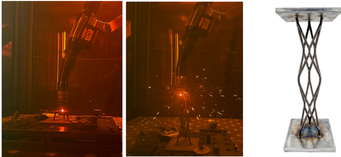
Fig. 6. Fabrication steps of a short 3-faced D-Pole.
