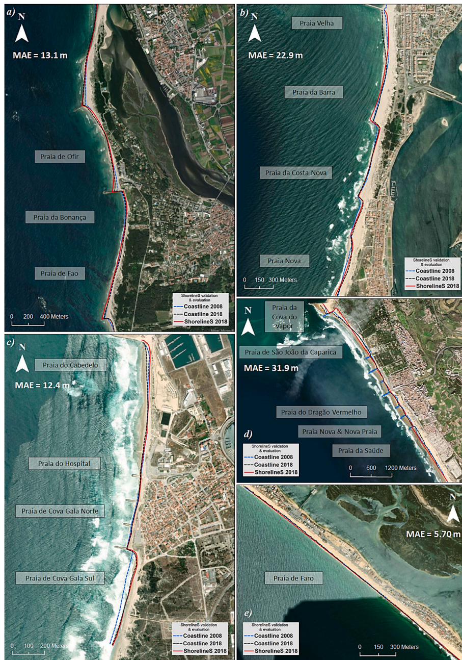
Fig. 4. (a) Ofir, (b) Costa Nova, (c) Cova Gala, (d) Costa da Caparica and (e) Praia de Faro observed shoreline (2008 – blue dashed line, and 2018 – black dashed line) versus modelled shoreline in 2018 from 2008 initial conditions, forced by the propagated-corrected-propagated ERA5 reanalysis (red line). Relevant locations as well as the areawide MAEs are overlaid.
