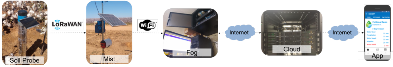
Fig. 4. SWAMP dataflow from infrastructure point-of-view
