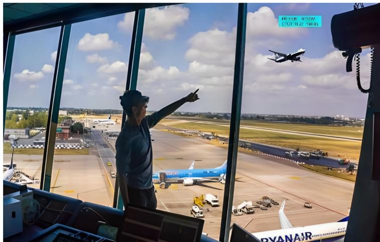
**Figure 1.** *RETINA* concept—an operator with the HMD and the displayed information seen superimposed through the window.
