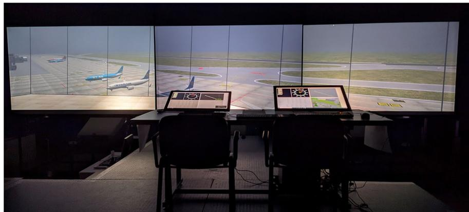
**Figure 2.** Validation platform implemented in the CAVE-like virtual environment of the University of Bologna.
