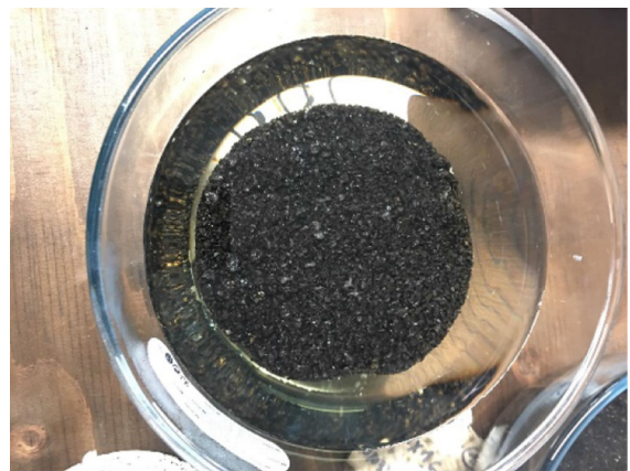
Fig. 4 Glass vessel containing the rubberised asphalt in direct contact with the water
