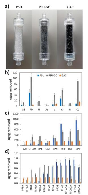
Fig. 3 a) PSU, PSU-GO and GAC cartridges and adsorption selectivity on b) heavy metals, c) organic contaminants, and d) PFASs.
