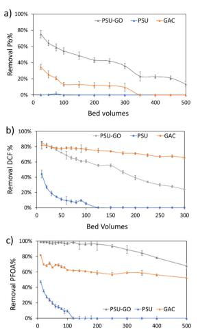
Fig. 5 Loading curves of a) Pb, b) DCF, and c) PFOA expressed as removal % vs. bed volumes of PSU (blue lines), PSU-GO (grey lines) and GAC (orange lines). Full results are reported in Fig. S15, ESI.†
