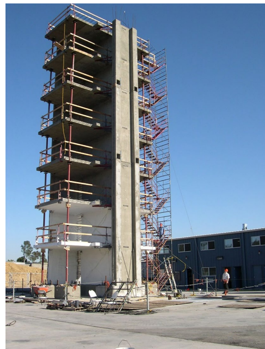
Fig. 6 Test structure: a slice of a seven-story RC wall building [32]
