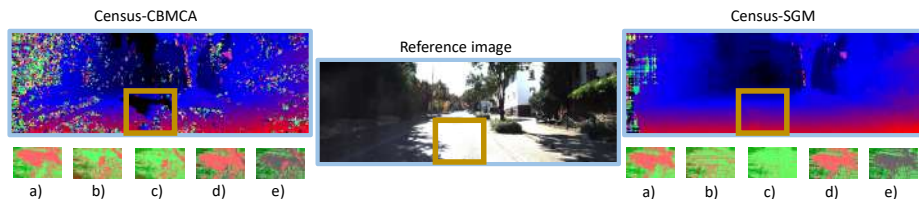
Fig. 2. Effects of different criteria. Given the highlighted region, we show inliers (green) and outliers (red) guesses by using the following cues in multi-modal binary cross-entropy: a) \mathcal{T}^p, \mathcal{T}^q b) \mathcal{A}^p, \mathcal{A}^q c) \mathcal{U}^p, \mathcal{U}^q d) \mathcal{T}^p, \mathcal{A}^p, \mathcal{U}^p, \mathcal{T}^q e) \mathcal{T}^p, \mathcal{A}^p, \mathcal{U}^p, \mathcal{T}^q, \mathcal{A}^q, \mathcal{U}^q . For black pixels, the considered configuration gives no guesses.
