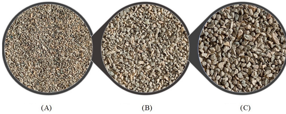
Fig. 1. Categorization of the selected recycled concrete grain sizes: 0.6–1 mm (A), 1–1.7 mm (B), 1.7–2.36 mm (C).
