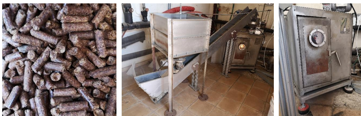
Figure 2. Pellets of dry brewer's spent grains (BSG), an overview of the pilot incineration plant and detail of the incineration unit.
