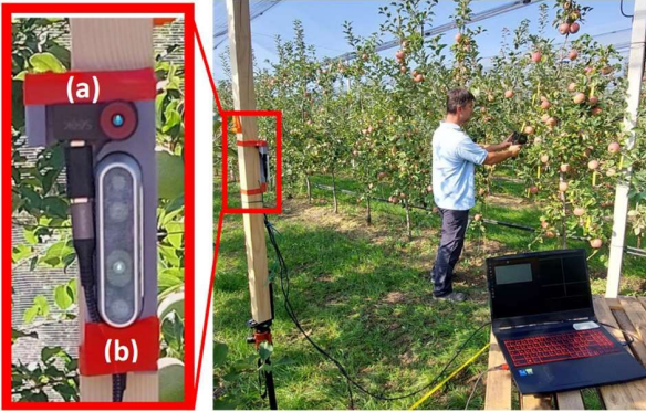
Fig. 1. Left) The 3D printed case holding (a) thermal camera and (b) RGB-D camera. Right) Platform sensors set-up and field data collection.
