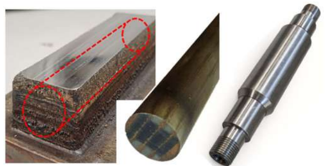
FIGURE 8. Fabrication sequence: as-built multilayer block, intermediate cylindrical preform, and finish-machined rotor.
