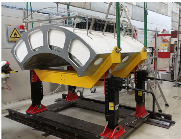
Fig. 17 The ENUBET demonstrator in the CERN T9 beamline. The white layer between the inner part of the detector and the SiPM electronics is the borated polyethylene shielding. During the test, only 20% of the detector (length: 80 cm, 18^\circ coverage in the azimuthal angle) was instrumented grouping the fibers and steering them to the SiPM boards located on top of the black plastic guides above the shielding. A test with an increase of the readout fraction by a factor 3 has been performed in August 2023
