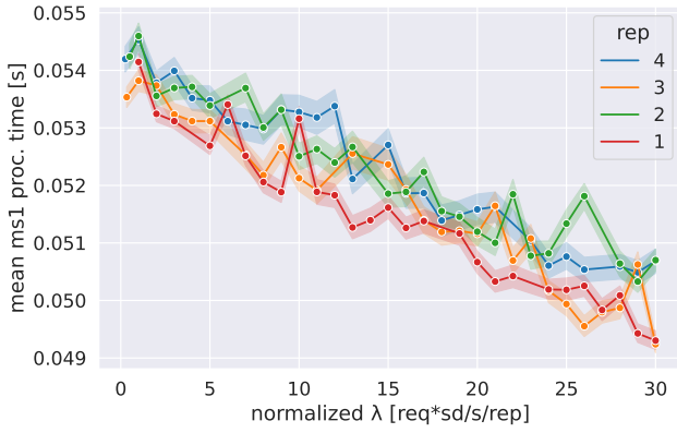
Fig. 5. Comparison of ms1 mean proc. time (95% confidence interval) for sd = 10x . The processing time is plotted for different combinations of RPS values and numbers of replicas. The RPS ( \lambda ) is equally balanced among replicas.
