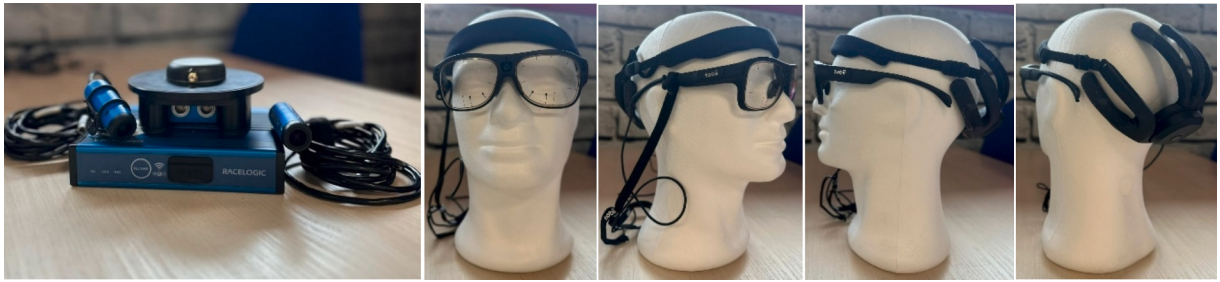
Fig. 3. Representation of Video V-Box and setting of Tobii Pro Glasses 3 and Mindthoot EEG on driver's head.
