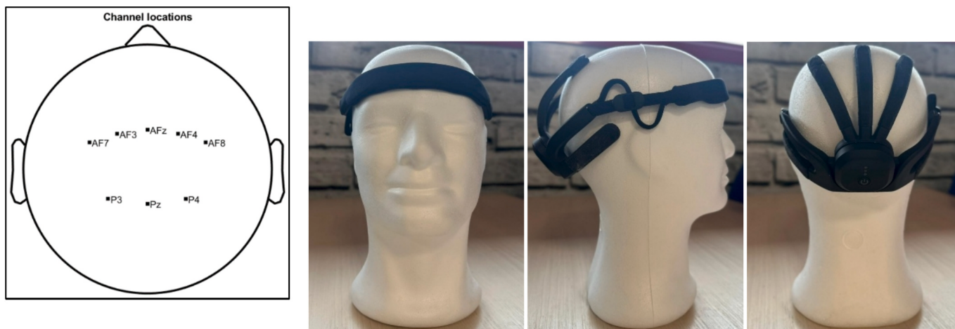
Fig. 4. Electrode placement in the Mindthoot EEG device, displayed through EEGLAB, and visual representation of the electrodes from Mindthoot EEGs positioned on a model human head.
