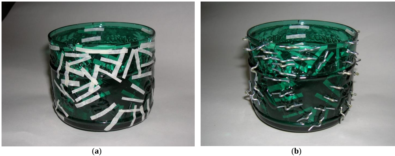
Figure 1. Application of paper tape stripes (a) and metal clamps (b) to the glass.
