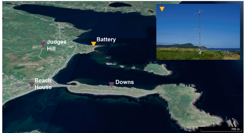
FIGURE 1 Southern view of Ferryland supersite area with the locations of the subsites: Battery (main site of this investigation), Beach House, Judges Hill, and The Downs. The flux tower, surface energy budget station, ceilometer, and visibility sensors at the Battery site are shown in the right-top panel. [Colour figure can be viewed at wileyonlinelibrary.com ]
