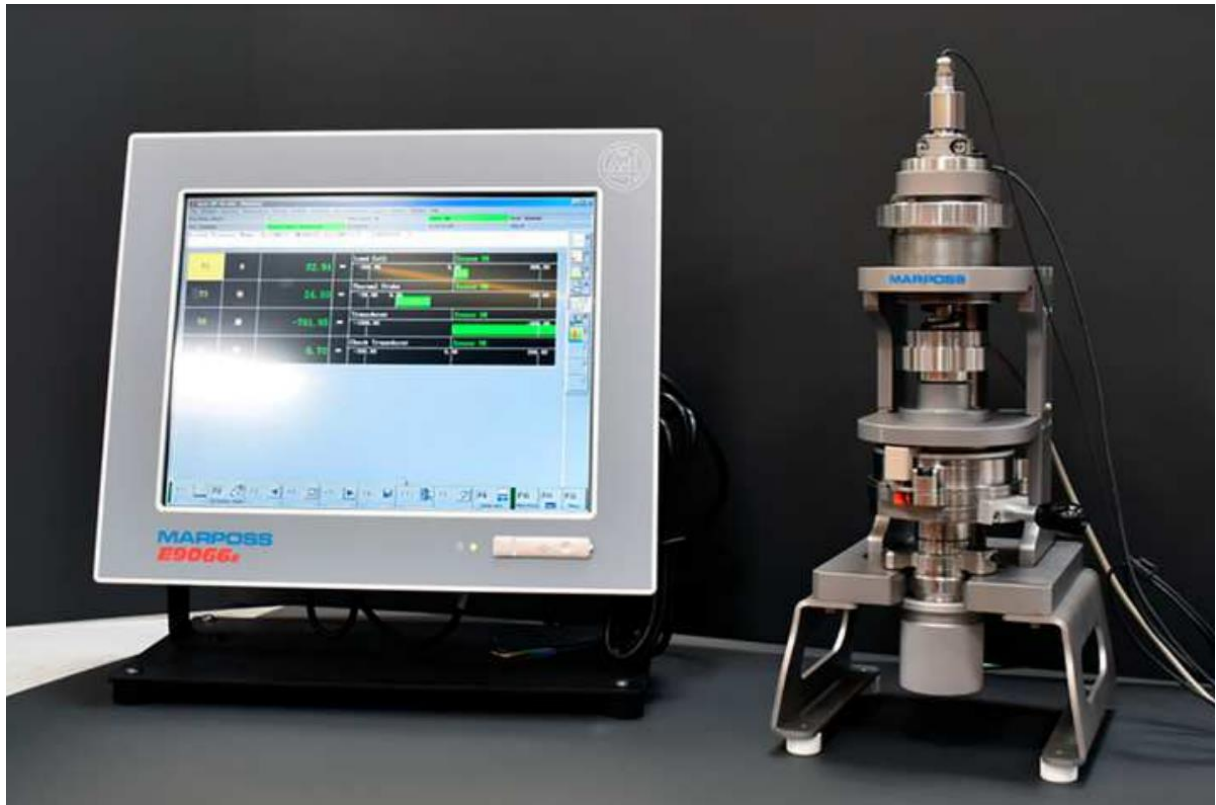
Figure 1. Marposs electrochemical dilatometer with electronic control unit.
