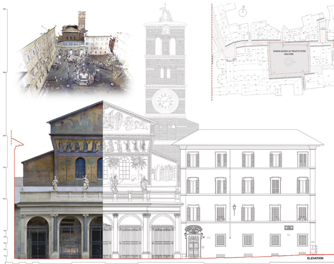
Example of the outcomes of the integrated survey of the Basilica of Santa Maria in Trastevere in Rome.
