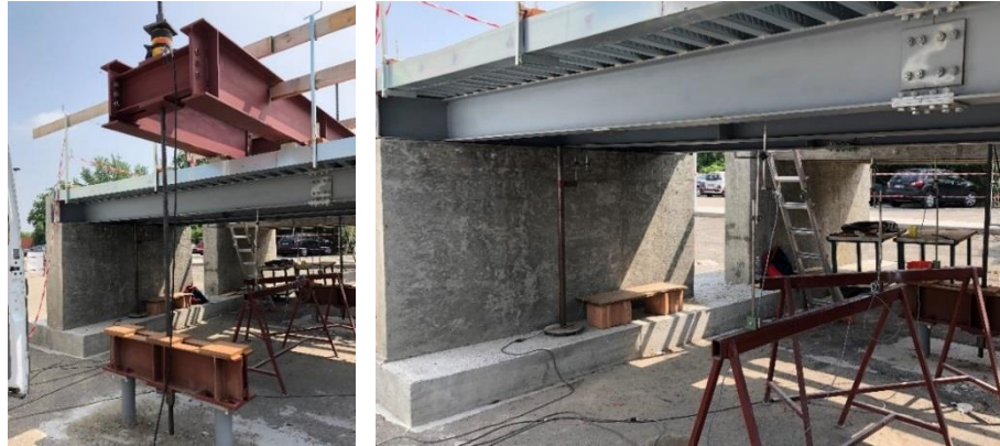
208 Figure 6: Static load test setup: on the left is shown the static loading system; on the right is 209 visible the data acquisition system.
