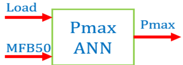
Figure 15. Calculation chain for Pmax.
