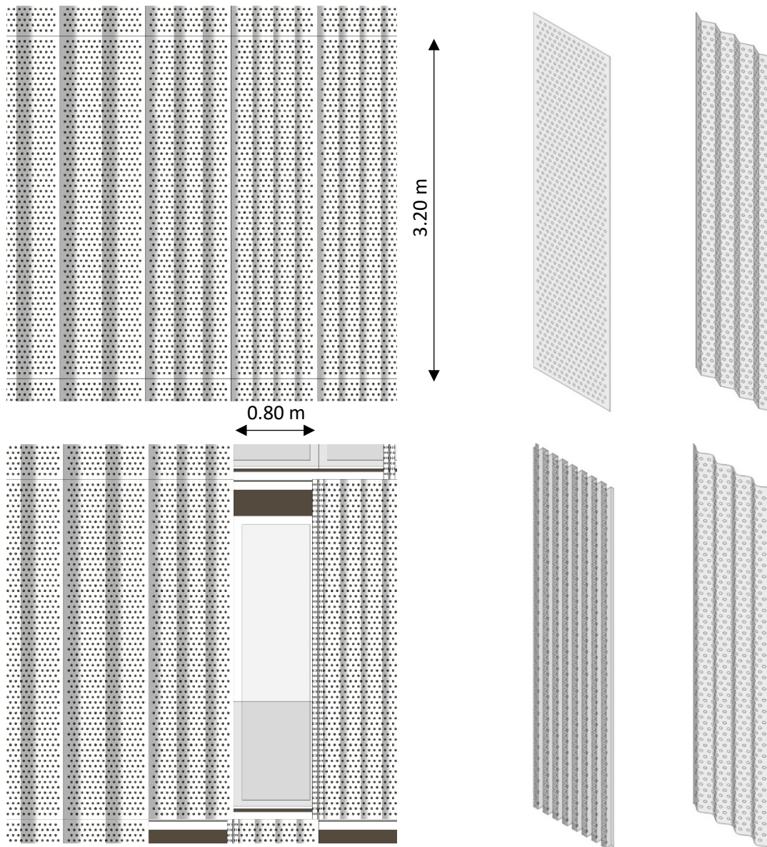
Figure 5. Layout drawings of the shading system and override position (bottom) with alternative panel sections from flat sheet to wavy sheet.
