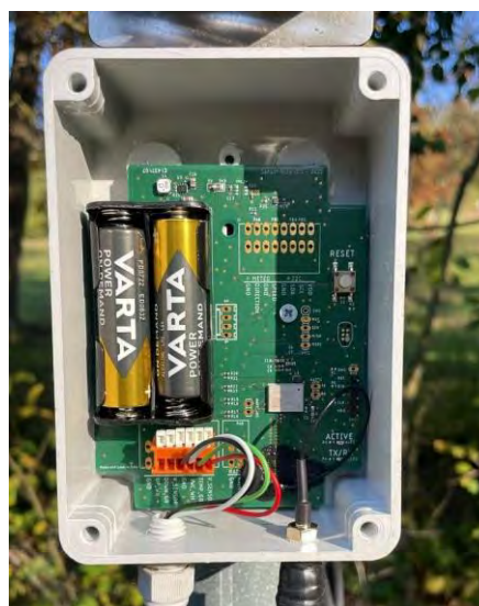
Fig. 2 - PCB integrating microcontroller and LoRa radio
