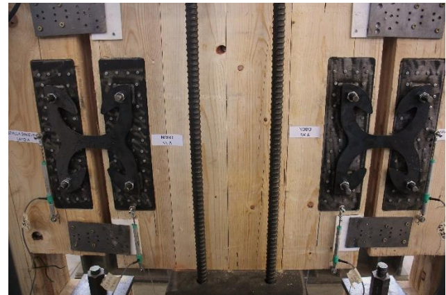
Fig. 2. Setup geometry (a) and instrument disposition (b) for NP and RNP fastenings.
