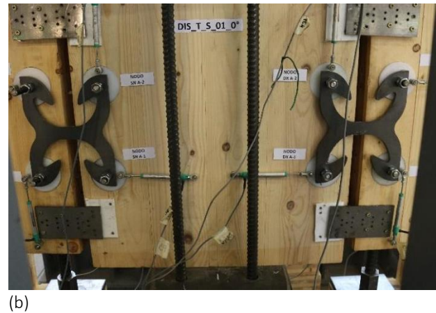
Fig. 2. Setup geometry (a) and instrument disposition (b) for NP and RNP fastenings.
