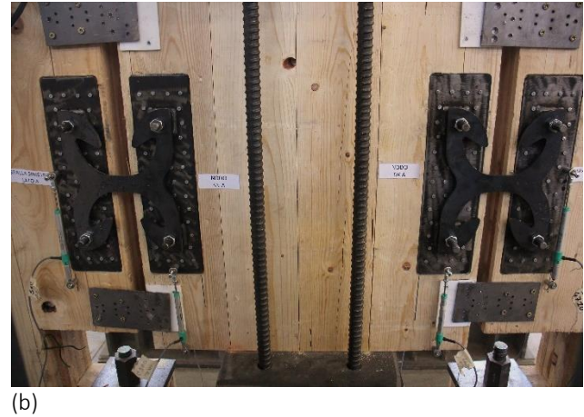
Fig. 2. Setup geometry (a) and instrument disposition (b) for NP and RNP fastenings.
