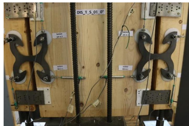
Fig. 2. Setup geometry (a) and instrument disposition (b) for NP and RNP fastenings.
