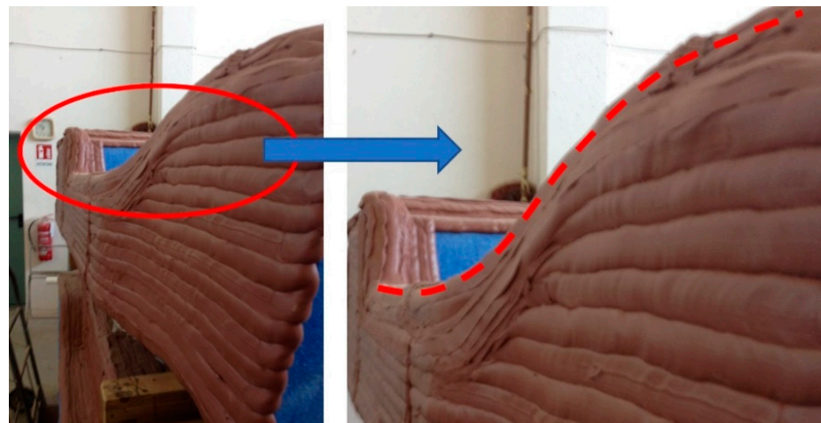
Figure 11. Modelling clay deposition along 3D paths over a large-scale mould for marine applications. On the right, a detailed view of the path followed by the extrusion head.
