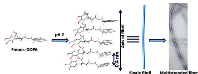
Figure 5. Schematic representation for the proposed model of self-assembly of Fmoc-L-Dopa at pH 2. Adapted with permission from ref. 34. Copyright (2013) Royal Society of Chemistry.
