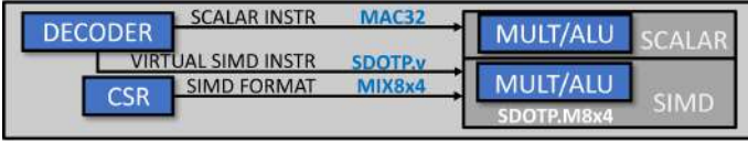
Fig. 3. Control signals for SIMD and Scalar instructions. The SIMD instruction is a Sum-of-Dot-Product, and the format is a mixed-precision 8x4. The bottom picture contains the encoding of the formats that are contained inside the CSR.
