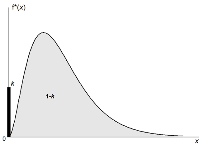
Fig. 4 Mixed probability distribution of flows with zeros. Zero values have a probability mass ( k ). The complementary probability ( 1-k ) of the non-zero values is represented by the probability distribution function, f^*(x)
