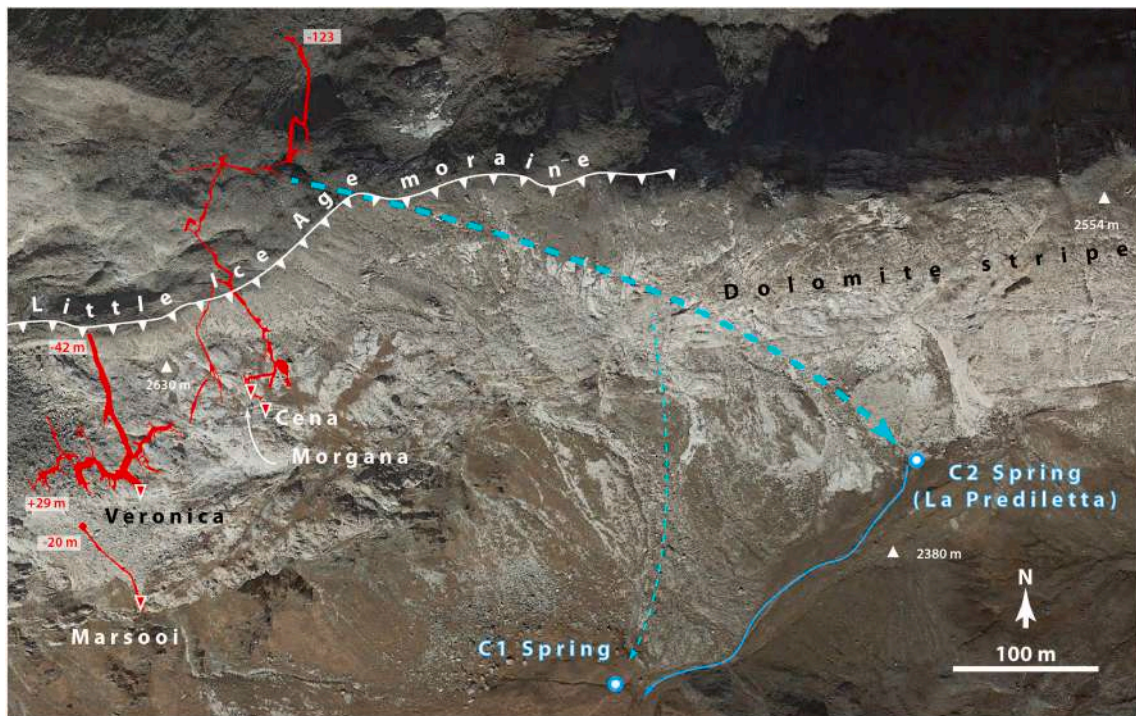
Fig. 9. Map of caves, injection point, water sampling points, and monitored springs during the dye tracing test. The E-W dolomite stripe outcrop appears in light colour across the center of the image. The light blue arrows show the hydrological connection. For position of C3 and C4 (out of this figure to the right) see Fig. 10.
