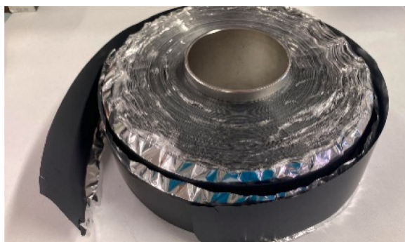
Fig. 1. The production roll scraps of the LiCoO 2 electrode.
