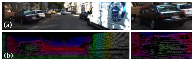
Fig. 7. Raw LIDAR for proxy supervision. We show a reference image (a) from the City domain alongside proxy labels sourced by raw Lidar (b), with the latter exhibiting wrong measurements at depth boundaries.
