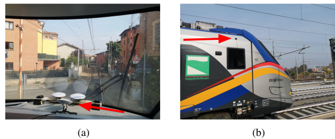
Fig. 5. Dynamic tests: Sensor node antenna measurement setup for Sensor Node 1 (a) and Sensor Node 2 (b)
