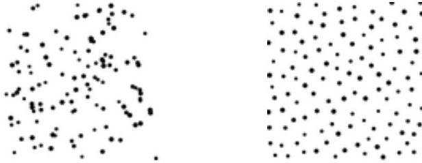
Figure 6.8: Two 100 x 100 pixel images with 122 random dots. On the left, the dots are selected from two random uniform distributions (one for each coordinate). On the right, the result from the application of the Bridson algorithm.
