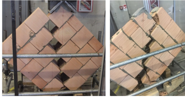
(a) (b) Figure 8: Diagonal compression tests on masonry walls: (a) typical rupture pattern; (b) rupture along clay blocks.
