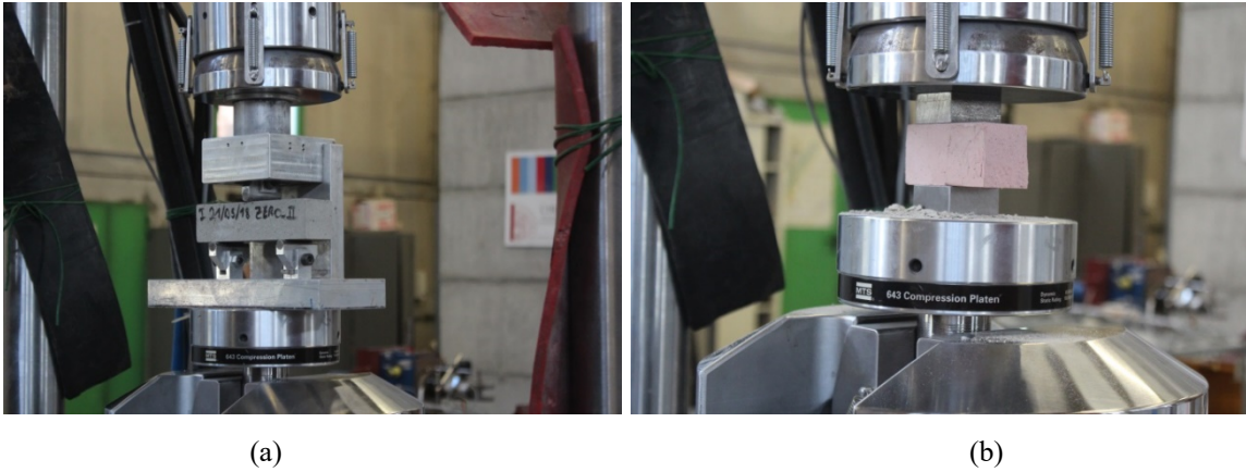
Figure 2: Experimental set-up for the mortar characterization (a) three-point bending test; (b) centered compression test.
