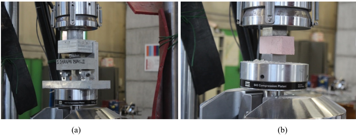
9 10 (a) (b) 11 Figure 2: Experimental set-up for the mortar characterization (a) three-point bending test; (b) centered compression 12 test.
