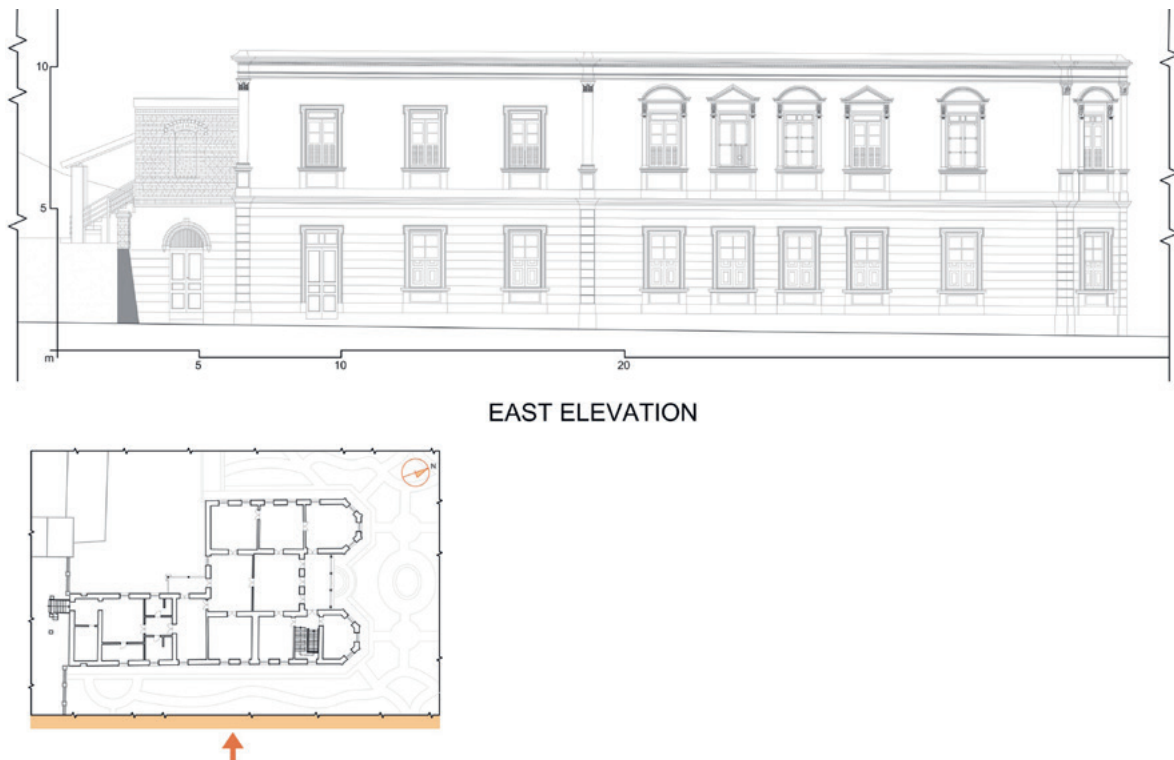
Fig. 9. 2D Drawings of the façades of the Casa Sede generated from the 3D survey. Source: Authors.
