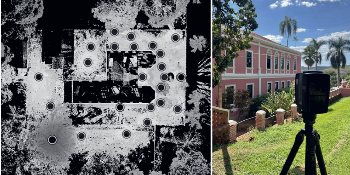
Fig. 8. Laser scanning process. Source: Authors.
