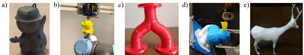
Fig. 14 Manufactured test parts from: a and b) Beam guided searching algorithm [18]; c) Cutting-plane algorithm based on overhang minimization [105]; d) Genetic algorithm [115]; e) Medial axis algorithm [100].
