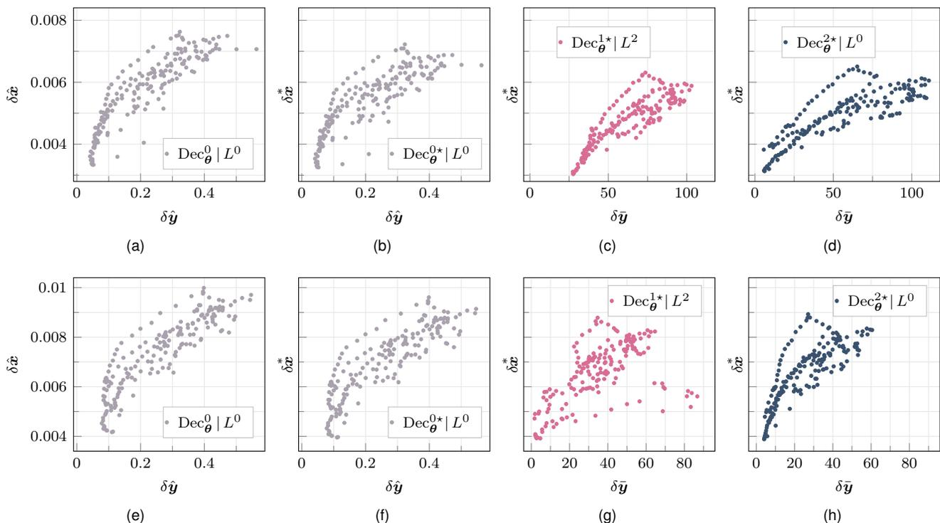
Fig. 7. Error in the measurement constraint fitting versus reconstruction error for the images composing the test set. Results are for all considered approaches except for  $\text{Dec}^{1*}|L^1$ . Top plots are for  $R = 4$  while bottom plots are for  $R = 8$ .
