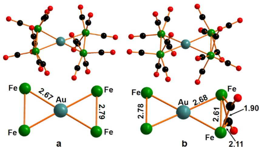
**Figure 3.** Upper part. Optimized structure of the: a)  $[\text{Au}\{\eta^2\text{-Fe}_2(\text{CO})_8\}_2]^-$  without bridging CO ligands and b)  $[\text{Au}\{\eta^2\text{-Fe}_2(\text{CO})_8\}\{\eta^2\text{-Fe}_2(\text{CO})_6(\mu\text{-CO})_2\}]^-$  with two bridging COs. Lower part. Simplified scheme of M-M distance and bridging ligands where available
