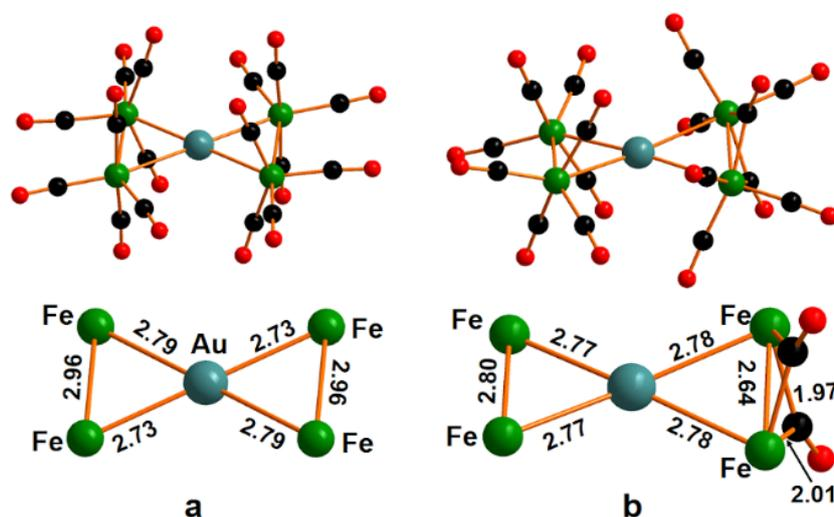
**Figure 6.** Optimized structure of the reduced form (in the upper part): a)  $[Au\{\eta^2-Fe_2(CO)_8\}_2]^{2-}$  without bridging CO ligands and b)  $[Au\{\eta^2-Fe_2(CO)_8\}\{\eta^2-Fe_2(CO)_6(\mu-CO)_2\}]^{2-}$  with two bridging COs. In the lower part, simplified scheme of M-M distance and bridging ligands where available.
