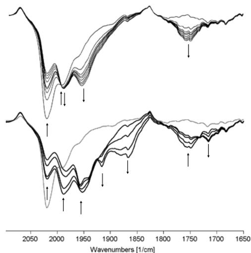
**Figure 1.** Infrared spectra recorded in an OTTLE cell during the stepwise overall reduction of  $[\text{Au}(\eta^2\text{-Fe}_2(\text{CO})_8)_2]^-$  ( $0.9 \times 10^{-3}$  M) in MeCN solution ( $[\text{NEt}_4][\text{PF}_6]$  (0.10 M) as supporting electrolyte). Top: first reduction:  $E_w$  from  $-0.40$  V to  $-0.60$  V, vs. pseudo-Ag electrode; bottom: second reduction:  $E_w$  from  $-0.60$  V to  $-0.75$  V, vs. pseudo-Ag electrode, grey line: initial spectrum.
