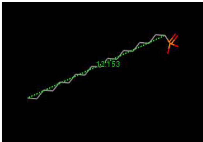
Figure S10 Structure of octadecylphosphonic acid molecule, the distance of carbon chain was measured by “Mercury” software is 12.153 Å
