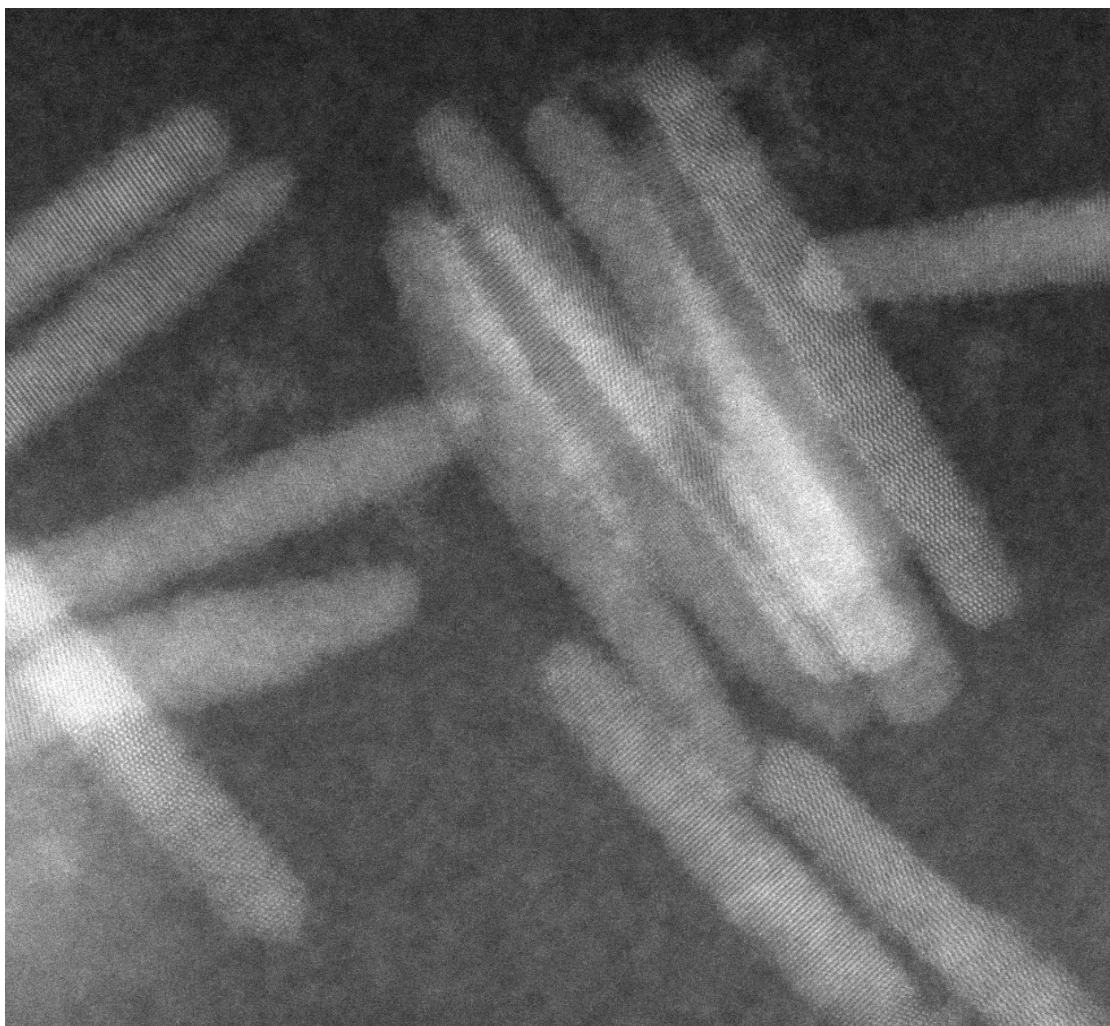
Figure S5 High resolution STEM of nanorods after 132 hours illumination. There was no trace of Ni cluster or particles on crystalline lattice of nanorods
