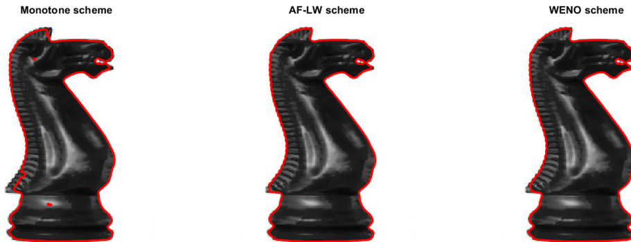
Figure 10: Test 3a with Datum 2. Plots of the final front using the monotone scheme N_i = 453 (left), the AF-LW scheme, N_i = 542 (middle), and the WENO scheme, N_i = 472 (right), with L^1 norm and tol = 0.00004 , \mu = 2 , K_{reg} = 5 , and velocity \tilde{c} .
