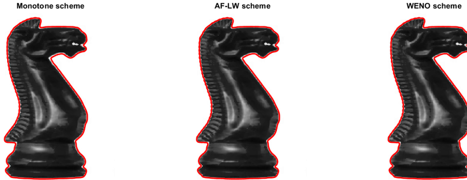
Figure 11: Test 3b. Plots of the final front using the monotone scheme (left), the AF-LW scheme (middle) and the WENO scheme (right) with velocity \tilde{c} , and tol = 0.00005 , by using L^1 norm in the stopping criterion and parameters \mu = 2 , and K_{reg} = 3 .
