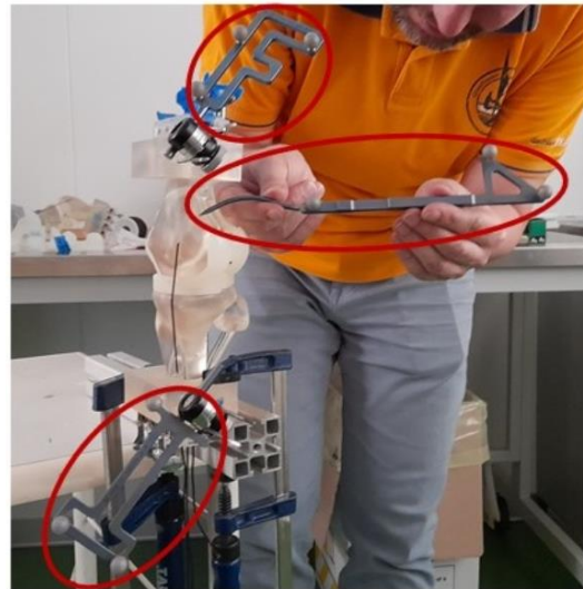
Figure 8. (a) Schematic representation of the camera distribution for the stereophotogrammetric system; (b) example of the experimental setup, in which the trackers and the pointer are enlightened.
