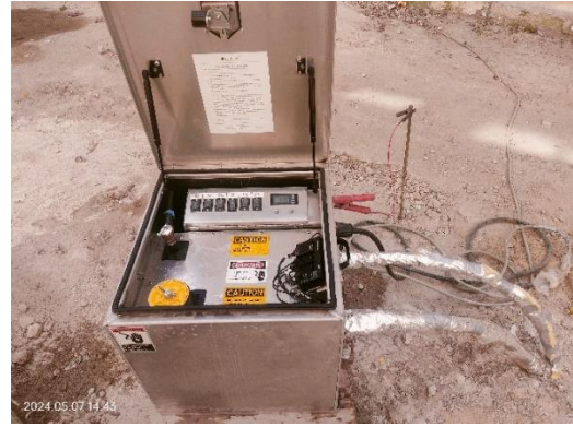
Figure 3: Carrying out onsite thermal response test on BHE-2.
