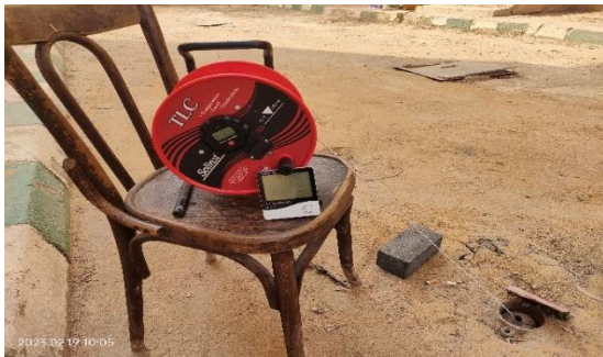
Figure 1: Measuring ground temperature in the piezometer during the exploration stage.
