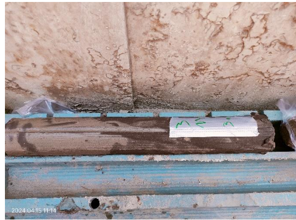
Figure 5: A sample collected from a drilled borehole for laboratory testing.
