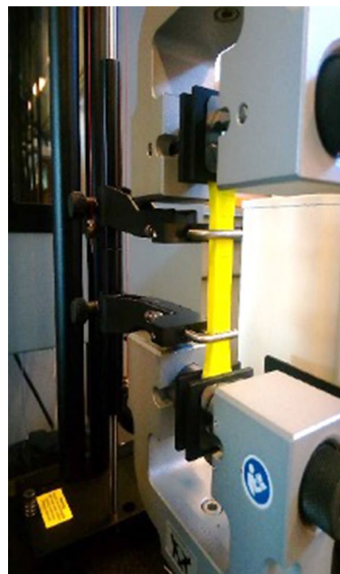
Fig. 2 Instron 3382 performing the tensile tests on a printed sample
