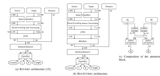
Fig. 2. Block diagram of our previous architecture (a), our novel architecture (b), and the attention block we use (c). The figure shows, next to each arrow, the dimensionality of the data involved, so as to clarify the size of the inputs and the outputs of each block. T is the temporal size of the data.
