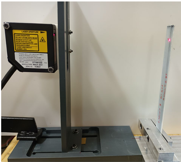
Fig. 6 Set-up used to test the cantilever beam to find the lamina Young modulus
