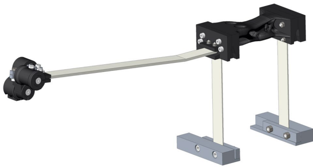
Fig. 4 Stephenson six-bar-linkage PRB model
