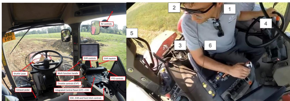
Fig. 3. UC1 Phase 1: real tractor used for testing (left) and users monitored by the proposed set-up (right) - 1 driver, 2 eye tracking glasses, 3 data storage unit, 4 CAN data recording, 5 GoPro camera, 6 biosensor
