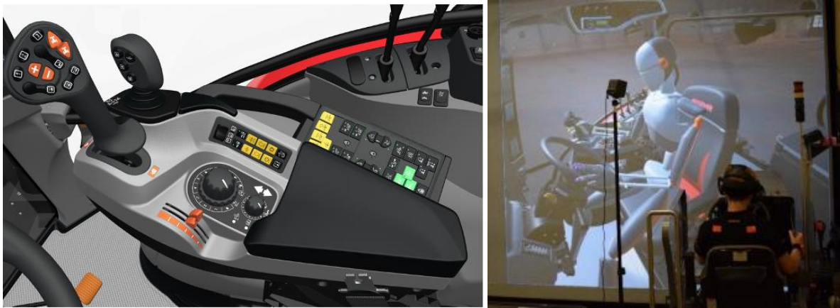
Fig. 6. UC1 Phase 3. Immersive VR test in Lab of the new armrest layout based on intuitive-grouped control panel
