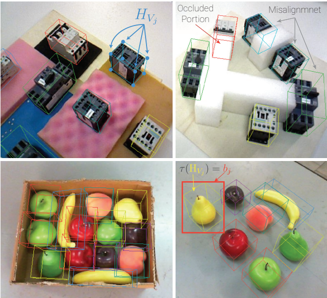
Fig. 3: Four random frames acquired during the creation of our new dataset: the first row refers to the Industrial dataset and displays virtual boxes drawn by the ARP; the second row shows samples from the Fruits dataset with annotations created off-line by the technique described in Subsection III-D.
